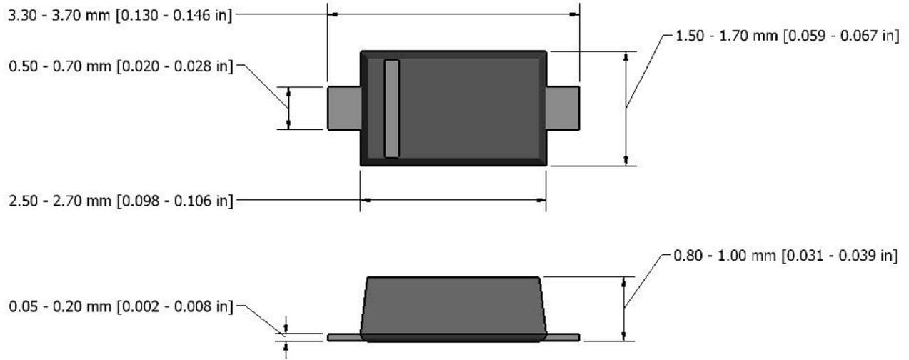
**Note:** Dimensions are exclusive of Burrs, Mold Flash & Tie Bar extrusions.
